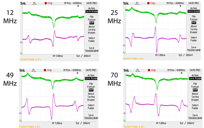
test wavelength: 671nm (Li-7 spectrum), rf in 20 dBm, error signal generated with phase detector ZRPD-1
