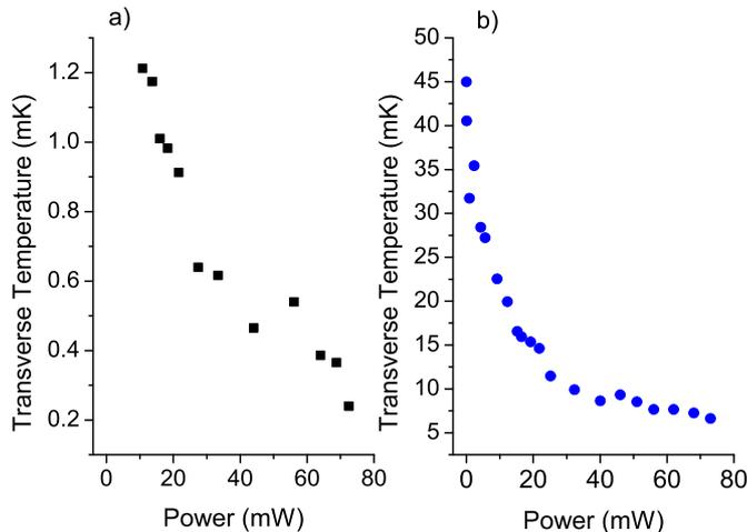
FIG. 7: Molecular beam temperature under a) Sisyphus and b) Doppler conditions as the power in the main pump laser is varied. Doppler cooling saturates at a main laser power of approximately 30 mW, while the Sisyphus cooling continues to increase as the power is raised. At powers below 10 mW, Sisyphus cooling is no longer observed.
