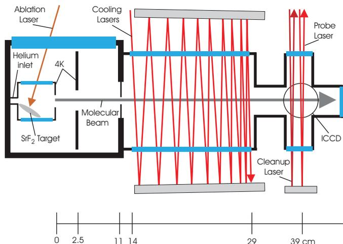
FIG. 4: Schematic of the experimental apparatus.
