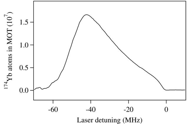
**Fig. 3.** Number of trapped atoms vs. detuning. The number of  $^{174}\text{Yb}$  atoms in the MOT is shown as the detuning of the laser is varied slowly from  $-60$  MHz ( $-2\Gamma$ ) to 0. The magnetic field gradient at the trap center was 75 G/cm. The number of atoms shows a peak at  $-42$  MHz or  $-1.5\Gamma$ . Other isotopes show identical behavior.
