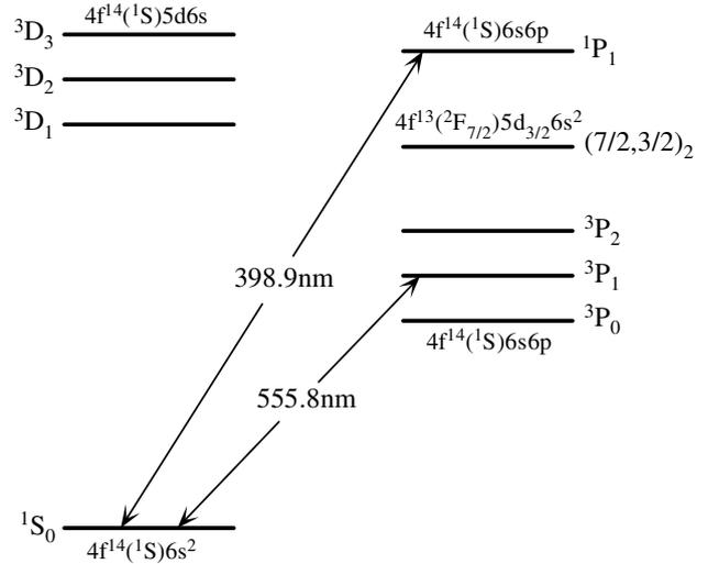
**Fig. 1.** Yb energy levels. The figure shows the relevant low-lying energy levels in Yb. Even-parity states are on the left and odd-parity states on the right. The two possible cooling transitions at 398.9 nm and 555.8 nm are shown.
