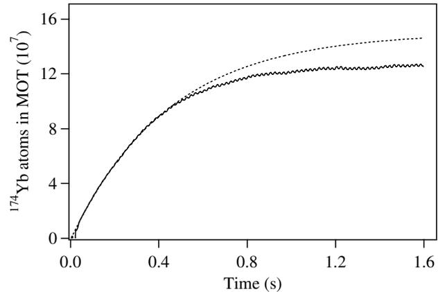
**Fig. 6.** Nonlinear losses. The number of  $^{174}\text{Yb}$  atoms in the trap (solid line) increases exponentially at first, but saturates at a lower value due to the  $N^2$  loss term in equation (1). The dotted line is the extrapolated exponential curve.
