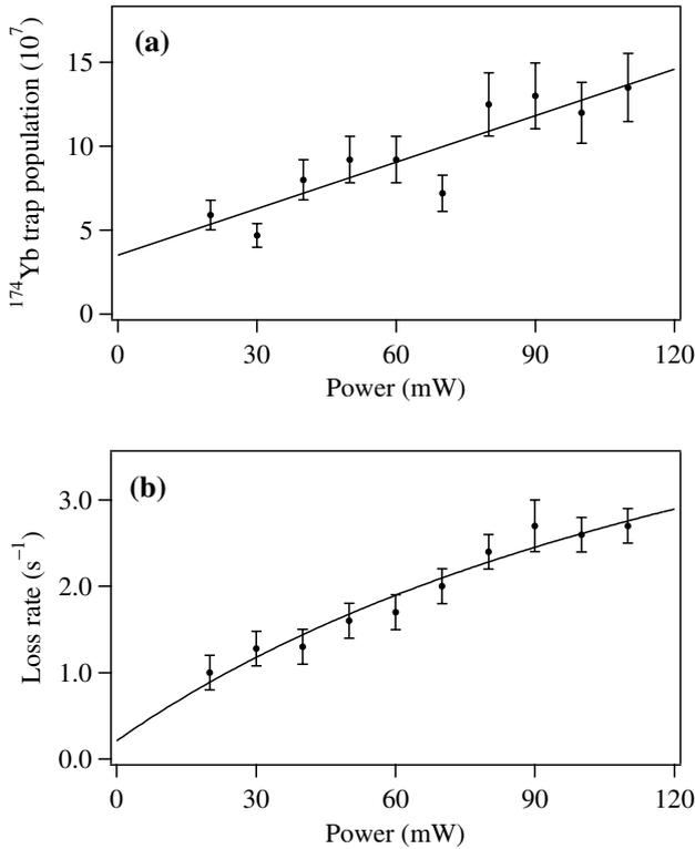
**Fig. 5.** Power dependence of the MOT. In (a), we show that the number of trapped  $^{174}\text{Yb}$  atoms increases linearly with trapping power. In (b), we study the loss rate as a function of power. The solid line is a fit to equation (2) in the text and allows us to separate the loss rates due to collisions and branching into metastable levels.
