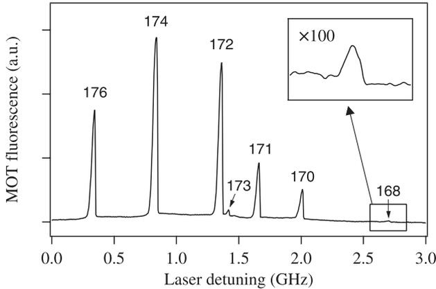
**Fig. 2.** MOT fluorescence vs. laser detuning. The fluorescence signal shows peaks as each isotope comes into resonance with the laser and is trapped in the MOT. Each peak is labeled by the corresponding isotope number. The inset shows a  $100\times$  magnified view of the region where  $^{168}\text{Yb}$  is trapped.
